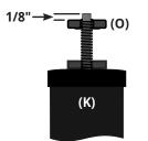
1. Loosen wing nut (O) on Black Berkey® Element (K) stem until the top of wing nut (O) reaches the top of stem's threads (about 1/8" from top end of stem).
